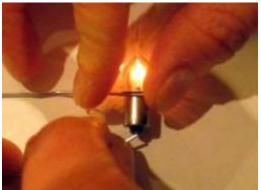
5. Observe how bright the lamp is when attached to a single battery. Just like in class, we will be scoring the brightness of the lamps on a scale of 0-10, where a score of 0 means the lamp is turned off, and a score of 10 is the brightest. This time, we will give the lamp connected to a single battery in the simple circuit a brightness score of "5" (see Table 1, below). This score will give you a baseline for comparison with the complex circuits.
