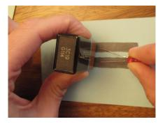
5. Try using only one pencil resistor and connecting the other LED terminal directly to the battery. See if you can slide the LED terminal back and forth along the resistor. (Warning: Do not connect the LED to the battery without a resistor – at least one lead of the LED must be connected to the pencil resistor at all times or the LED will burn out.)
