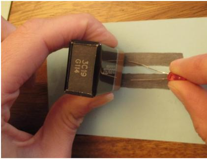
5. Try using only one pencil resistor and connecting the other LED terminal directly to the battery. See if you can slide the LED terminal back and forth along the resistor. **(Warning: Do not connect the LED to the battery without a resistor – at least one lead of the LED must be connected to the pencil resistor at all times or the LED will burn out.)**
