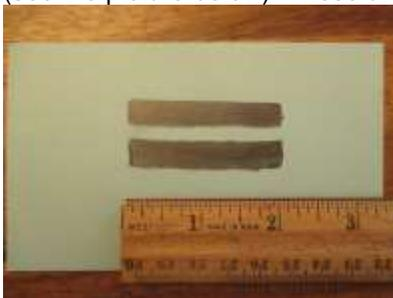
3. Place the battery on the two pencil resistors so that one battery terminal is on each resistor. Pay attention to which rectangle is touching the positive terminal and which is the negative. (The positive terminal is marked with a “+” on the side of the battery.)
