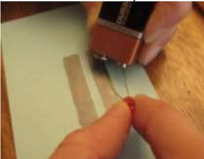
6. If you have a multimeter, you can use it to measure the resistance along the resistor. Follow the instructions that came with your meter and see how the resistance is related to the length of the resistor.
